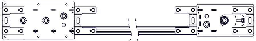
Fig. 5: Installation variants – Single-track system with motor mounted on the left and deflection unit mounted on the right
